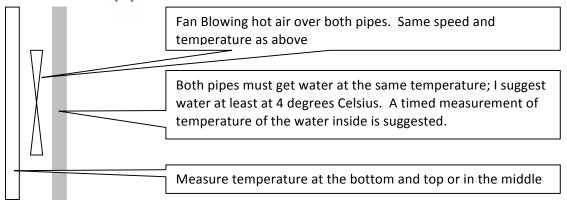
Marius, note, that infrared or surface temperatures will give you the wrong indications. It is important to measure the water temperature in the pipe. Ideally, the temperature should be taken in the centre of the pipe.
